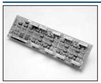
The MCN-8 uses 8 consecutive addresses on the METRA-BUS thus allowing up to 8 MCN-8s to be connected to a single METRABUS driver board. Reading each of the addresses will return the current count of that channel. Writing to a counter causes the counter to be cleared.
